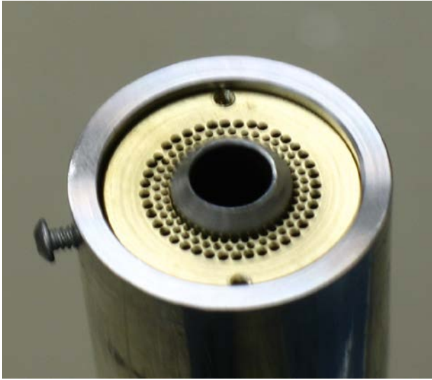
Fig. 1 - Details of the straight burner setup: (a) Burner exit with sharp edge and perforated plate for the pilot flame tests, (b) Syngas conical flame stabilized with the CH 4 /air pilot flame.
