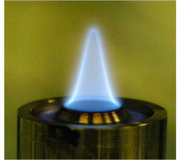
Fig. 1 - Details of the straight burner setup: (a) Burner exit with sharp edge and perforated plate for the pilot flame tests, (b) Syngas conical flame stabilized with the CH 4 /air pilot flame.
