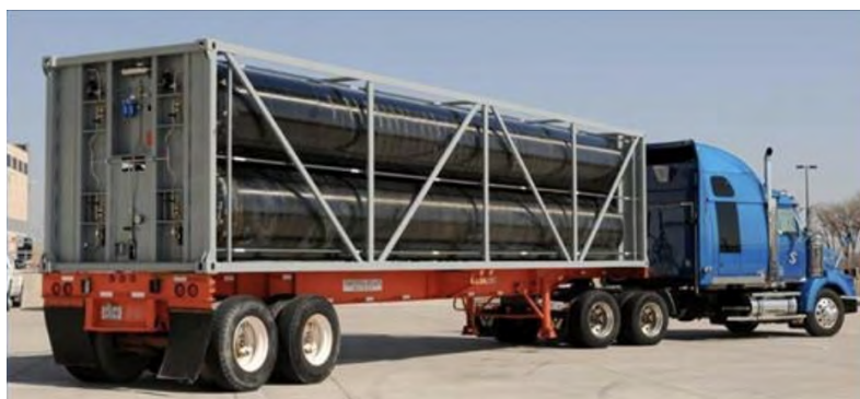
Photo: Composite tube trailer capable of delivering 550 kg of hydrogen at 250 bar lvii .
