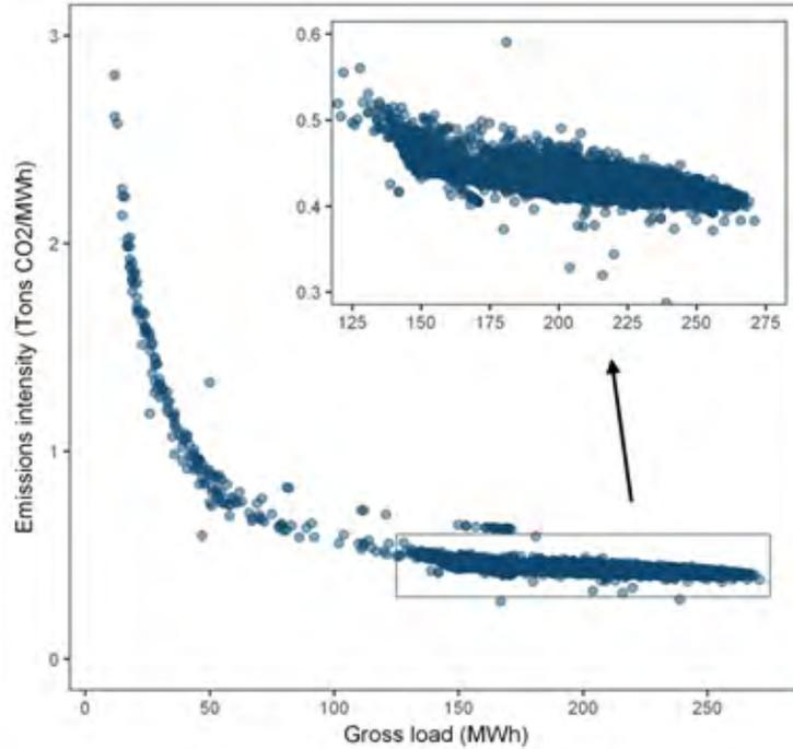
Figure 7: Observed annual emission intensity variation for a sample OCGT plant in California
