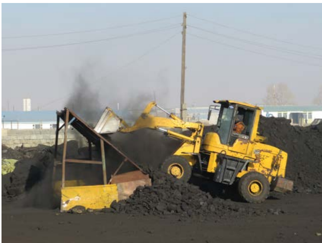
Coal sorting yard, where trains deliver coal into the city, and it is sorted by size and loaded on trucks.
