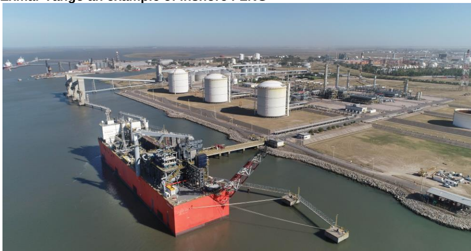
Figure 5: Exmar Tango an example of inshore FLNG
